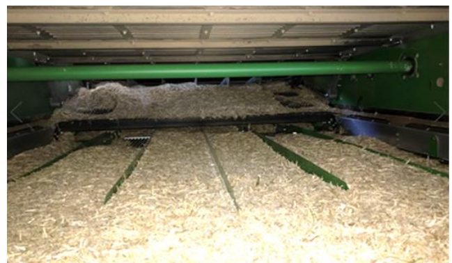
Same field, same condition with grate covers and optimized settings, notice reduced chaff on chaffer and more exposed dividers
